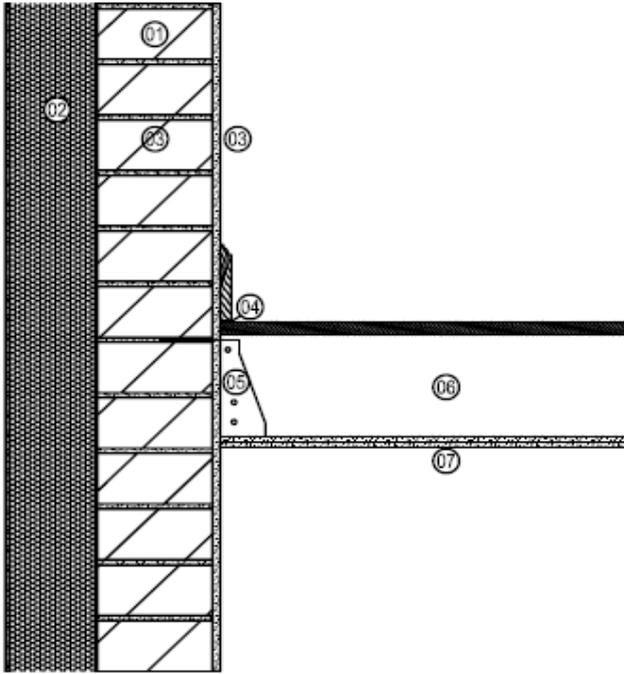
1. 215mm solid concrete block wall
