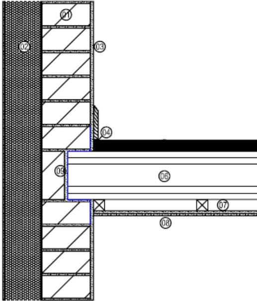
1. 215mm solid concrete block wall
